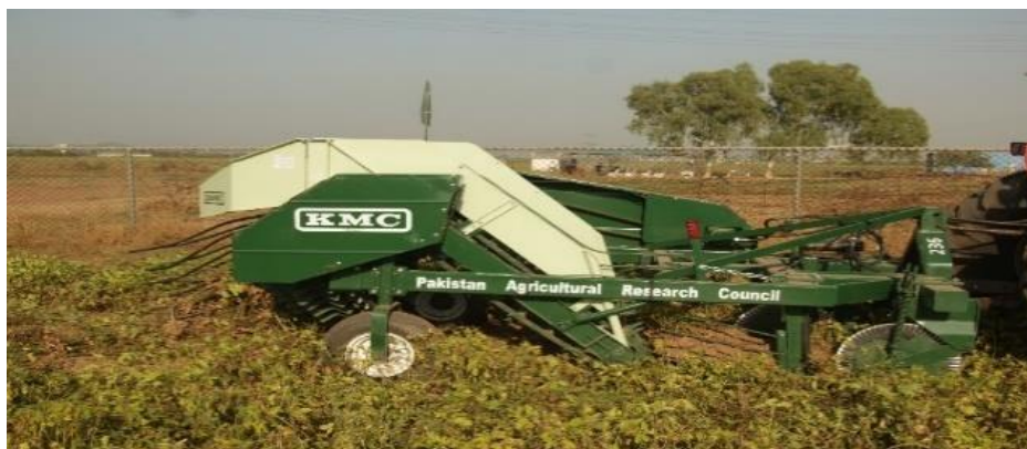
Fig 2. KMC 2-row groundnut digger-inverter
