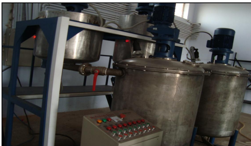
Fig. 35: Machinery for preparation of bio-pesticides
