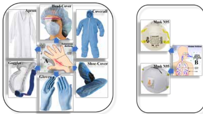
Fig.1 PPE for protection against A. Cutaneous and B. Respiratory route of infection
